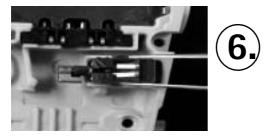
Step 9. Place the vibra assembly into its slot. Use tweezers.
